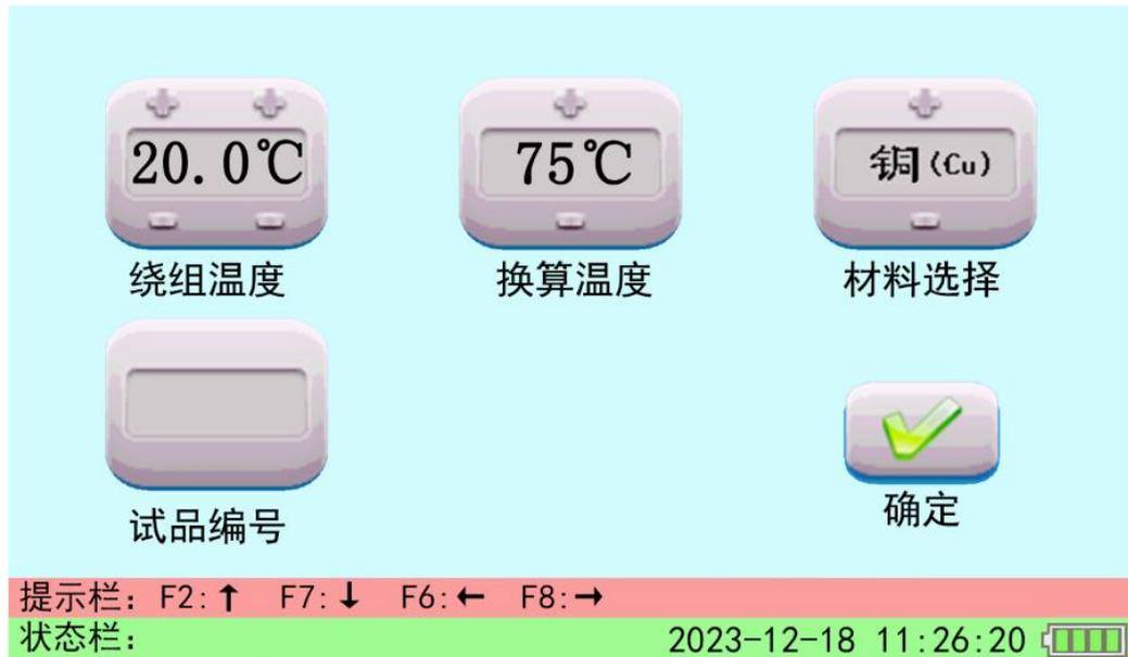
**Winding temperature:** the current temperature of the tested article;
