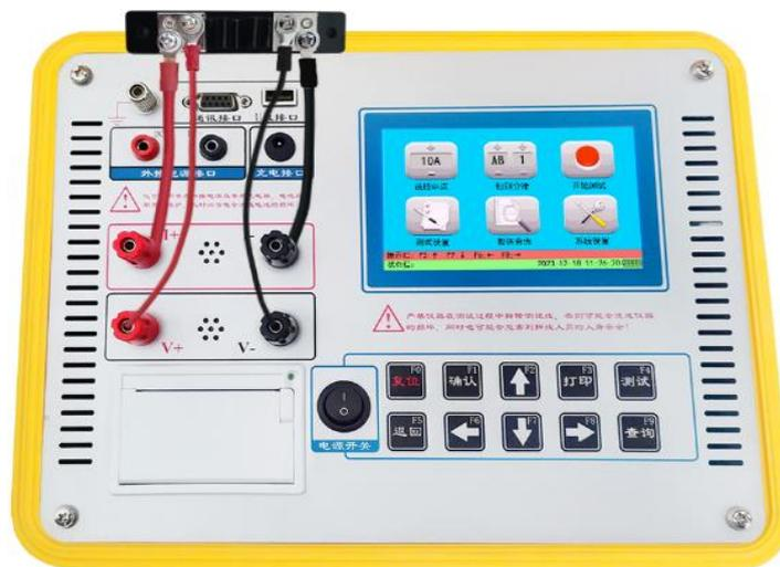
Test the resistance value of the standard resistance according to the normal test steps. If the test result complies with the resistance value indicated on the standard resistance (within 0.2% error), the instrument is in normal condition and can continue to be used.
