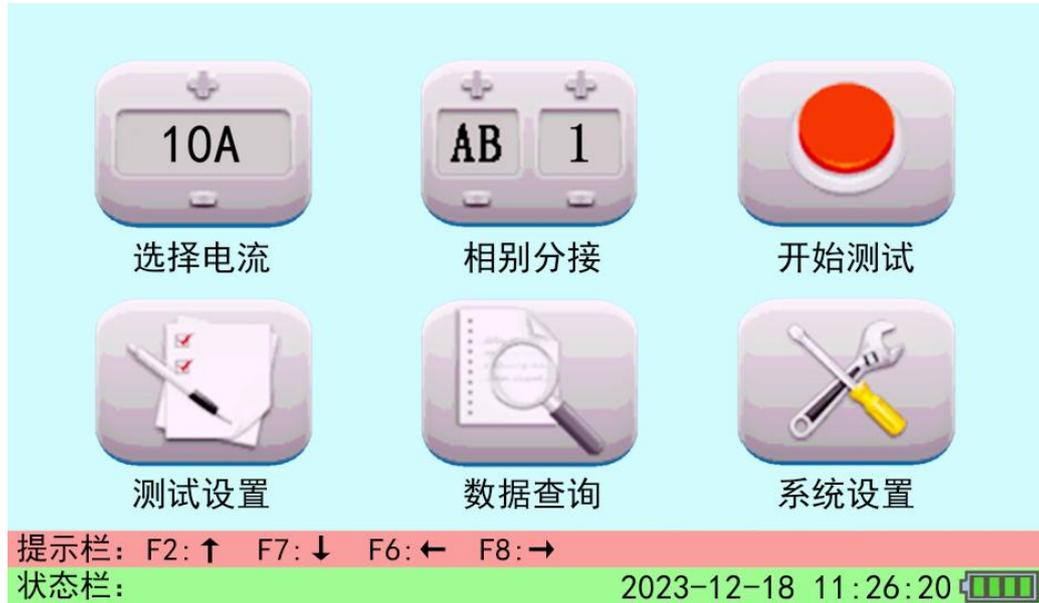
By touching the + - on the icon, select the desired current and select the tap and tap to be tested. (Also by key operation).
