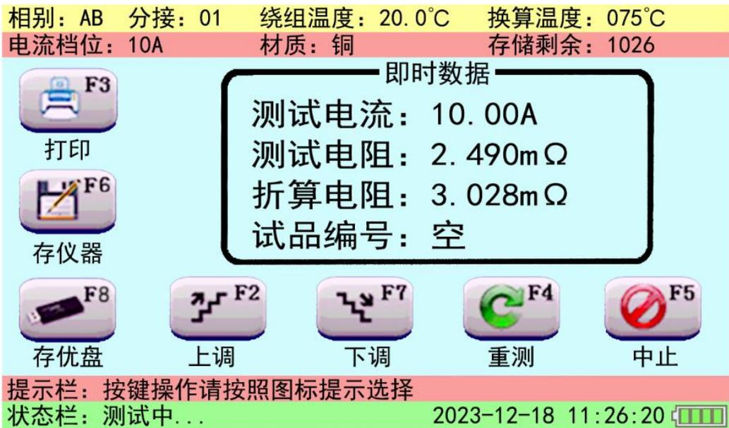
After a while, the status bar shows "in test...", indicating that the charging is finished and the test state is entered. Wait for the electromagnetic balance, the data is stable, can be read.
