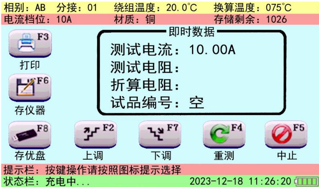
The status bar in the lower left corner of the screen shows "charging", and the "test current" of the instant data shows the current value through the test article.
